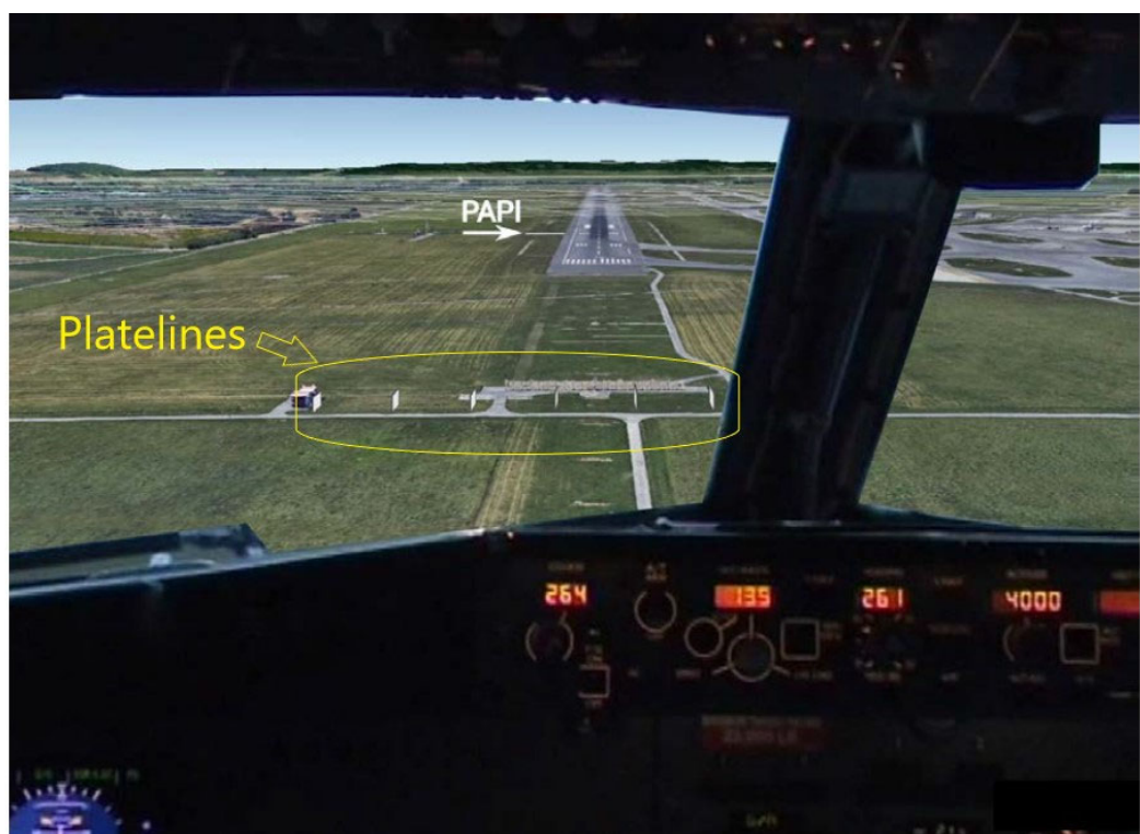
Fig. 1: Simulated view on the 400 M plate line array on final approach to runway 16
